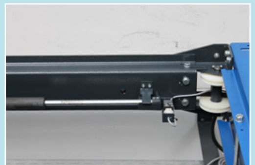
Electrical safety device to avoid contact with crossbar
