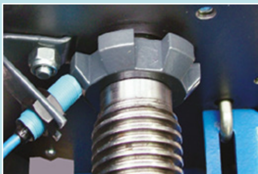
Wear and maintenance-free proximity switch for non-contact height measurement
