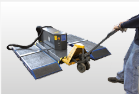
The lift can be moved using a conventional dolly or forklift thanks to the mobile frames. The lift requires no anchoring to the floor, the installation frame is self-supporting and only requires a solid ground surface..
