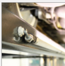
Rotating LED lighting for easy adjustment of light direction for glare-free vision.
