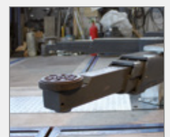
123 mm drive-over height on the support disc
