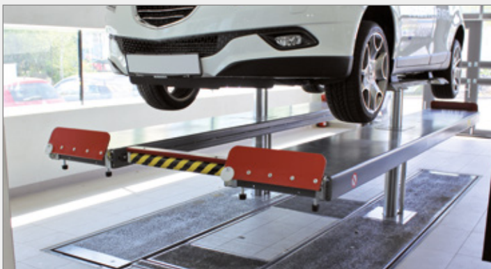
Setting of wheel-free jack or wheel inspection from the side
