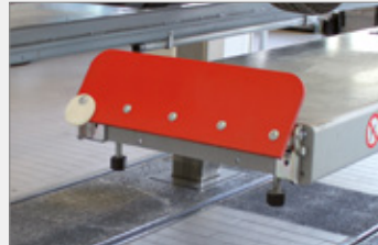
Automatic folding roll-off protection
