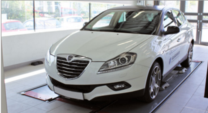
Lowered, making it easy to drive on with low ground clearance
