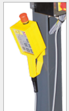
Mounted on pillar
