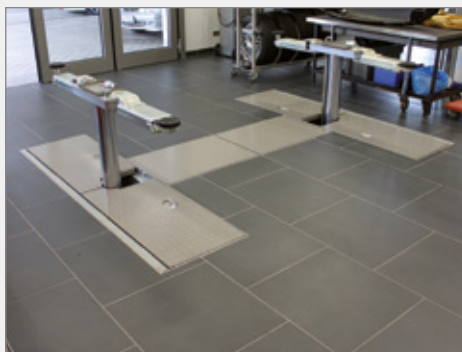
Opening and closing of the cover is supported by a pneumatic damper system
