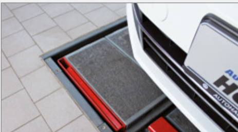
The floor compensation under the runway is a second ground surface, which levels off the surface below the lift.
