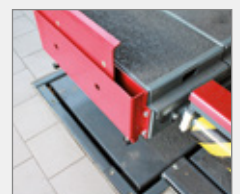
The floor compensation creates a uniform workshop floor.
