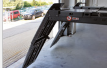
Folding drive-on ramp for high runways or low drive-on angle
