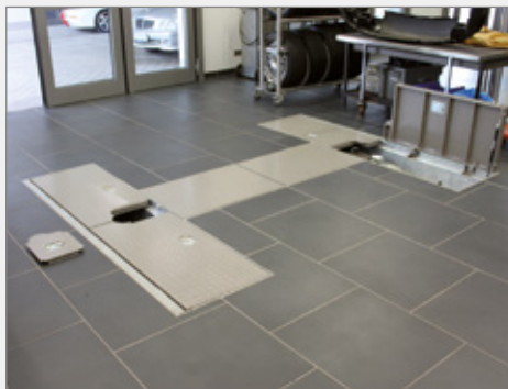
Opening and closing of the cover is supported by a pneumatic damper system
