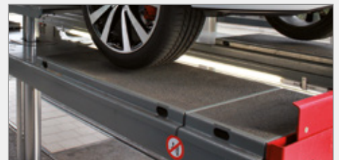
Runways with compensating plates for level adjustment to wheel-free jack or wheel alignment.
