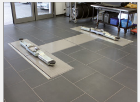
With closed covers, the lift can be used as a standard lift.
