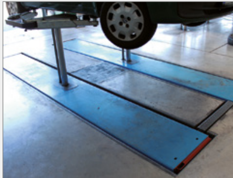
Runway lifts with integrated secondary lift (1860 mm) and high value wheel-free jack.
