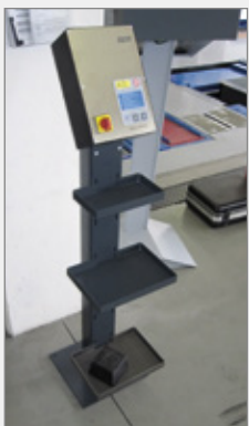
Control assembled on a control desk pillar, for installation as required
