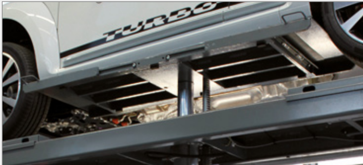
Runway lifts with platform wheel-free jack, sill support, load capacity: 3.5 t
