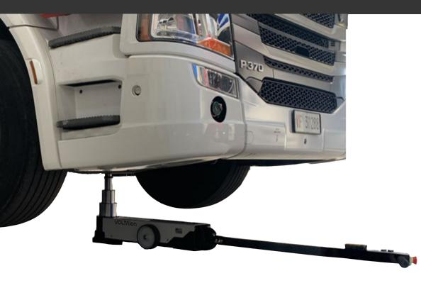
The motor-free descent utilizes the vehicle's weight, saving energy and time. You can choose Gravity Down or Control Down.
